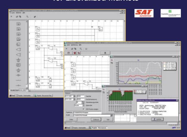
The energy management system SAT PROPHET includes the resource planning system (RPS) and the graphical topology editor (GTE). It has been developed for energy supply companies with combined heat and power generation and offers coordinated cost optimal planning of the power station park and the energy import from external companies. Modern forecasting and optimization techniques are used for the solution of this problem.
