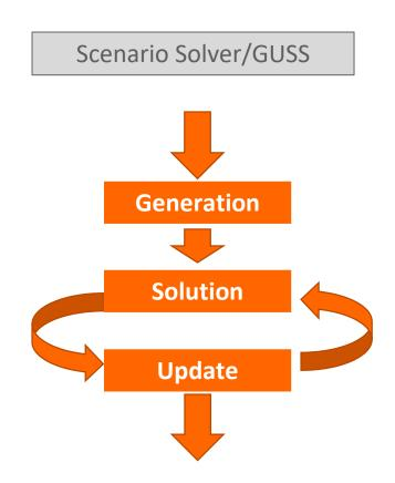
Generates model once and updates the algebraic model **keeping the model "hot"** inside the solver.
