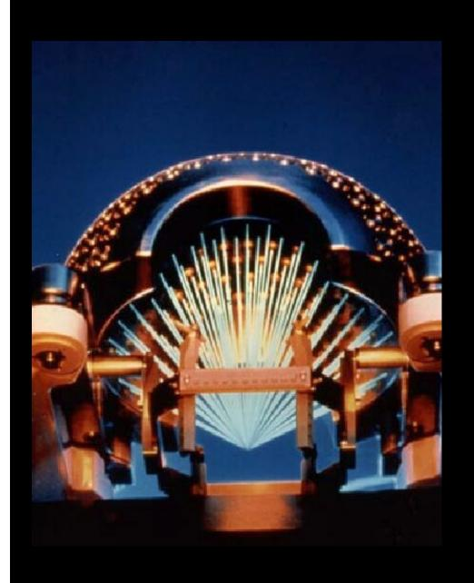
201 cobalt gamma-ray beam sources are arrayed in a hemisphere and aimed through a collimator to a common focal point.
