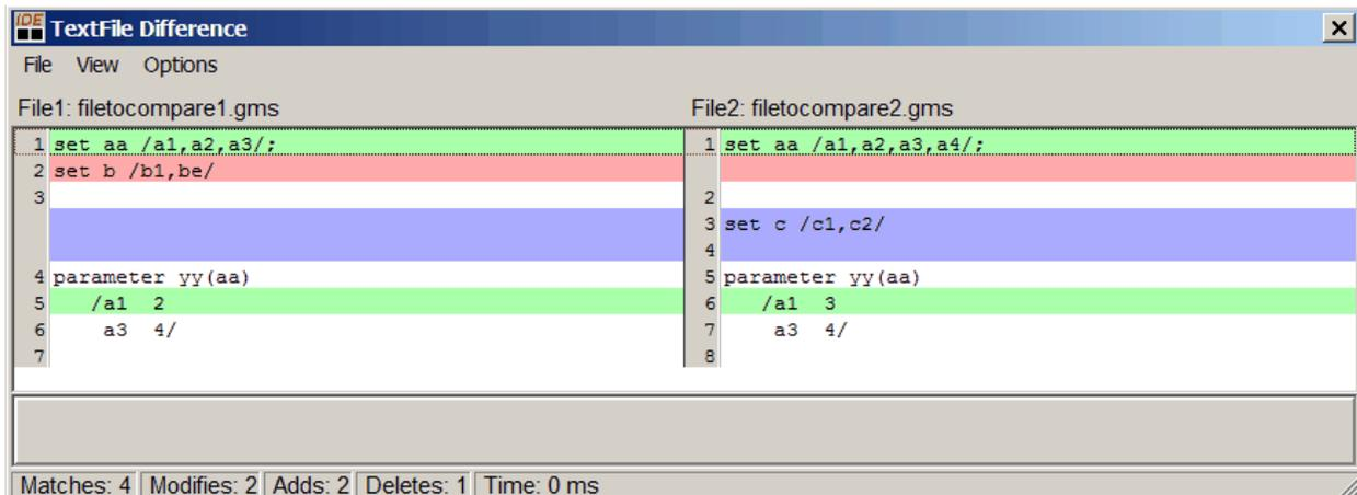
When lines are identical in both files they come out with a white background. Green lines identify those with differences in the line content. Reddish lines identify new lines in left hand file while blue identifies new content in the right hand file.
