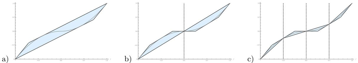
Figure 3: a) Polyhedral outer approximation of  $f \mapsto f |f|$ , b) initial spatial branching on zero, c) further spatial branching.
